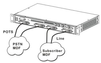
Figure 4-4 Rear Panel RJ-21 Connector Cabling for NCT480
